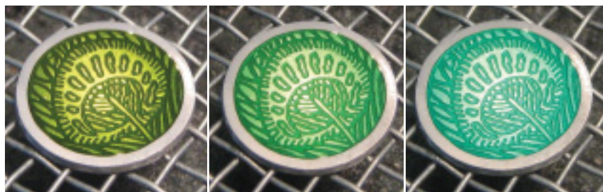
Images of a silver sample piece cooling down (l to r) showing how much the colour changes in the process
